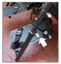
3 To adjust the depth position of the footrest, loosen the bolt on the tube that runs from front to rear
