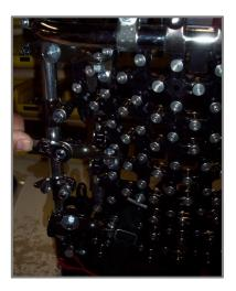
4 Loosen the Lynx nuts in the area you would like to adjust. Work methodically in either rows or columns. Once loose, pull the Lynx out or push it in until you obtain the required shape. Tighten the Lynx nuts, again working methodically in rows or columns to ensure they are all tight. Repeat the process as required.
