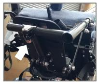
You can check the footrests are at the same height and centrally aligned by checking the tubes that run side to side are pointing towards each other.
