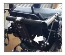
4 To adjust the width position of the footrest, loosen the bolt on the tube that runs from side to side
