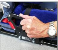
3 Use a tape measure to measure a fixed point on the seating system to ensure the backrest is square to the seat base.
