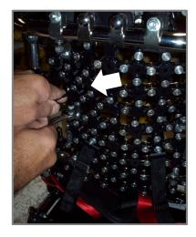
2 Loosen the bolt that runs through the backrest in a similar way. You may need to do this with the client out of the seat.
