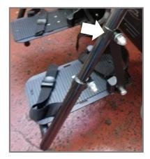
2 To adjust the height of the footrest, loosen the bolt on clamping the footrest vertical tube.
