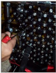
Remove the Evazote spacers and place the seat cushion back into position. If the shape of the backrest has changed significantly you will need to consider if a new backrest cushion is required. One may be required if it:
