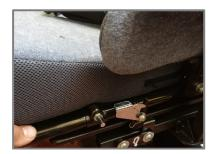
5 Standing at the side, hold the front carry handle and the rear of the seat, lift the seat unit off the interface board.
