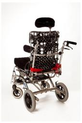
A Lynx Seating System has a special backrest whose shape can be changed over time. This can be to accommodate changes in posture. It consists of a number of interlinked plastic components. This will typically be fitted to the backrest of the seating system. The seat in the photo above is shown with the backrest covers and cushion removed.
