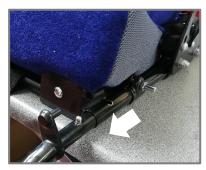
On some footrest types, like a padded footbox, both footrest drop tubes are linked together. If this is the case, you will need to release one side slightly, release the opposite to allow the complete footrest to be removed.
