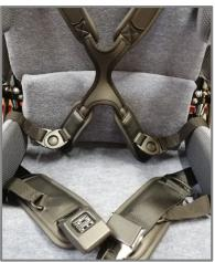
3 Disengage the two catches, one on each side of the seating system.
