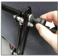
The backrest pivots with a Gas Strut controlling how easy it is to push. A Limiter limits the range of movement. The Lock enables the dynamic element to be removed when it is not required or should not be used, such as during transport.
