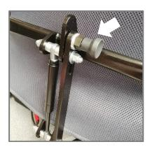
2 Disengage the lock to allow the dynamic backrest to move. Pull the Lock towards you and rotate it a quarter of a turn.
