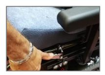
4 Holding the front of the seat, lift it out of the catch and put the front of the seat back down just in front of the catch.
