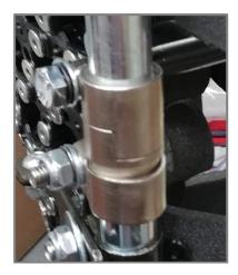
2 Lift the lateral support using the black tube attached to the pad. Lift it near the swingaway mechanism.
