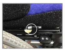
3 Slide the seat forwards and up to remove the seat.
