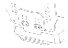
3 Locate the tongue in the slot. When the backrest is in position, it should be fully engaged.
