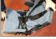
5 Both lugs at the front of the seat should engage on top of the framework.
