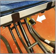
4 Adjust the seat to the required level of tilt. Reengage the tilt safety lock.
