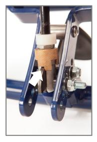
3 Fully support the seat and release the foot lever by pushing down.
