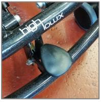
4 Adjust the seat to the required height. Reengage the safety lock.
