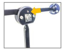
To adjust the angle of the headrest at the headrest end, loosen the bolts retaining the ball joint. Adjust the headrest to the required position. Tighten each of the three bolts equally.
