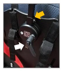
2 Adjust the stop sleeve (yellow arrow) to the top of the headrest socket and tighten the grub screw. This ensures that if the headrest is removed, it can be repositioned back into the same location.
