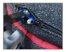
Using a 10mm ring spanner, loosen the joint and adjust to the required shape We recommend you only adjust one joint at a time. Ensure the bolts are fully tightened to avoid slipping out of adjustment.
