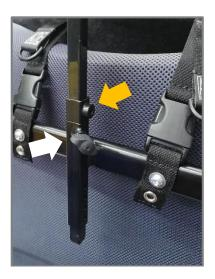
2 Adjust the stop sleeve (yellow arrow) to the top of the headrest socket and tighten the grub screw. This ensures that if the headrest is removed, it can be repositioned back into the same location.
