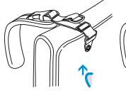
The Top Pull harness has the buckle mounted directly on the top of the pad. Fine adjustment is achieved by pulling the webbing from the top. The top mounting can be positioned anywhere on the backrest.
