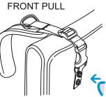
The unique Front Pull harness has a curved ladderlock buckle at the top of the webbing path. The webbing is easily pulled through from the front. The quick-release mounting can be positioned near the top of the backrest.
